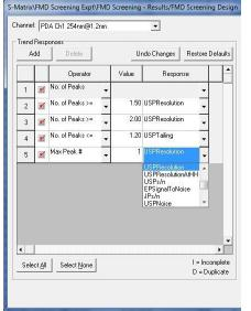
**FMD**'s patented Trend Responses eliminate the requirement for laborious and error-prone peak tracking in initial screening experiments. Flexible Trend Response operators enable you to automatically retrieve data for any separation characteristics you want to evaluate. Example Trend Responses which FMD can instantly obtain from all experiment chromatograms include:
