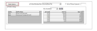
Maintain target level in each run: the software can maintain the target OLP variable in a given run (injection) as an absolute constant within the mobile phase independent of the change in the Strong/Weak solvent ratio across the gradient.
